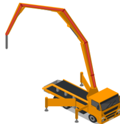
Concrete pump machine
